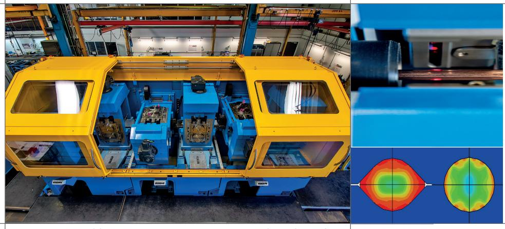
A complete range of Octogonal and Round Wire Reduction ROLLING MILLS
